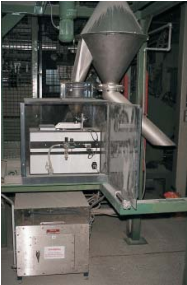
HAVER-CPA Online Unit equipped with roto sample divider and sample collector as used in the chemical industry.
